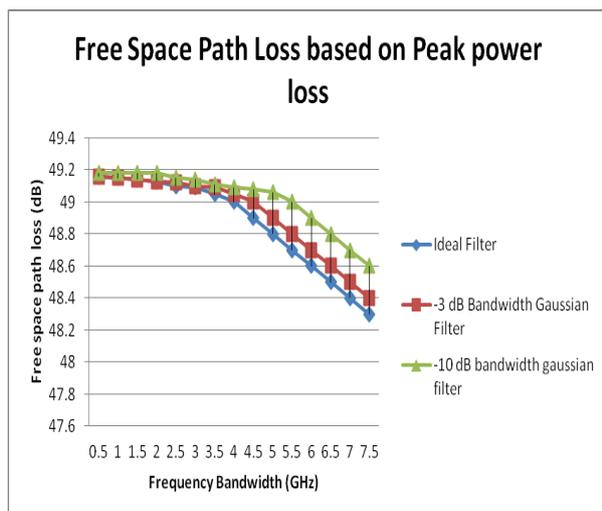
**Fig.9 Free space path losses based on peak power loss with centre frequency is  $f_c = 6.85$  GHz and T-R separation distance is  $d = 1$  m along frequency bandwidth  $f_b$  from 500 MHz to 7.5 GHz.**
