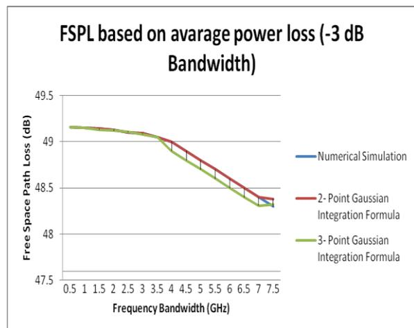
Fig.7 Free space path losses based on average power loss with centre frequency is  $f_c = 6.85$  GHz and T-R separation distance is  $d = 1$  m along frequency bandwidth  $f_b$  from 500 MHz to 7.5 GHz.
