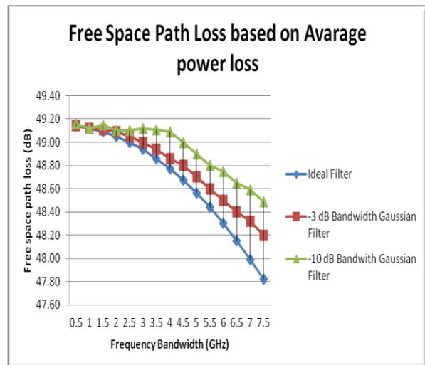
Fig.6 Free space path losses based on average power loss with centre frequency is  $f_c = 6.85$  GHz and T-R separation distance is  $d = 1$  m along frequency bandwidth  $f_b$  from 500 MHz to 7.5 GHz.
