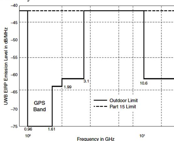
Fig.1: FCC spectrum mask for UWB [1]
