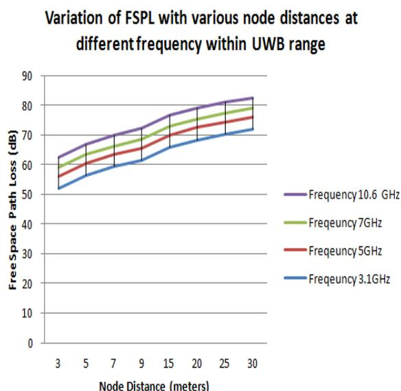
Fig. 11: Variation of FSPL at different frequency range and distances between transmitter and receiver
